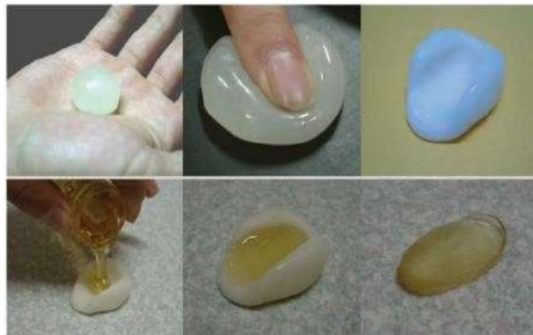
Figure 1 : Making an artificial fingerprint directly from a live finger plastic is used to obtain the mold and gelatin to obtain the cast.
